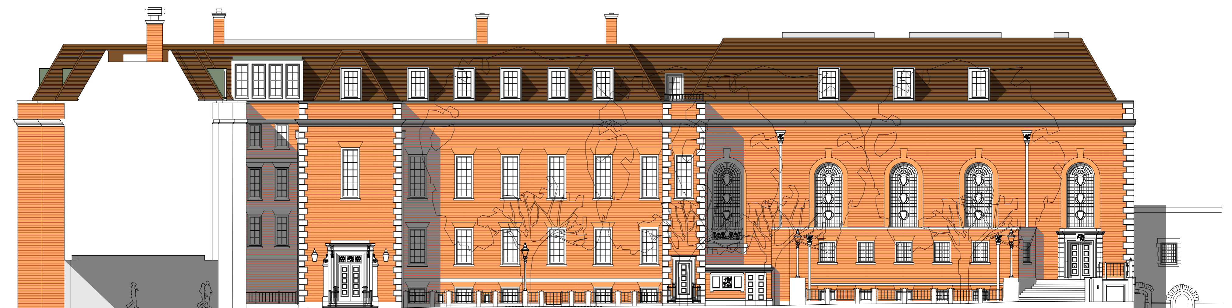
Proposed north facing elevation showing the mansard roof extending across the Hall and Treasury and the new lift shaft and escape stair.
